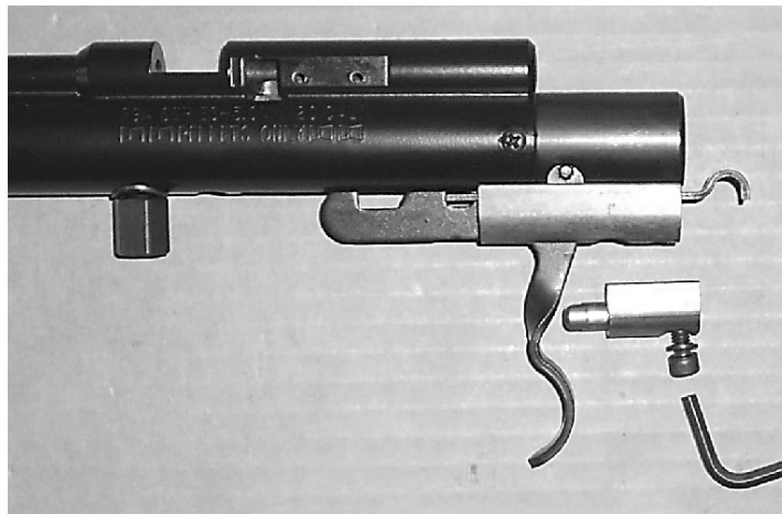
remove trigger spring components
