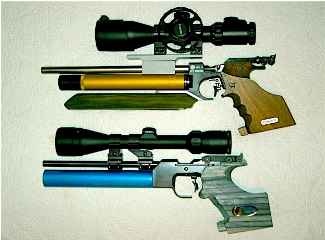
*The Steyr LP-1 illustrates a problem encountered when scoping most ten-meter guns; vertical-opening loading levers require very high scope mounts. One reason I've put up with so much Tau Mk 08 aggravation is the fact their **side-lever** loading allows much lower scope mounting for the lower centers-of-gravity and tighter trajectories I prefer.*
