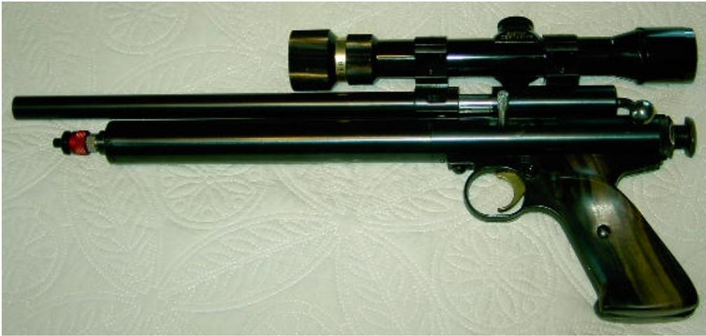
*As received, this .50 pistol produced 640 FPS on the first shot and 550 FPS on the second. After a re-seal and much de-tuning, it now returns 2 consistent shots per charge at 579 FPS with 181 grain balls.*
