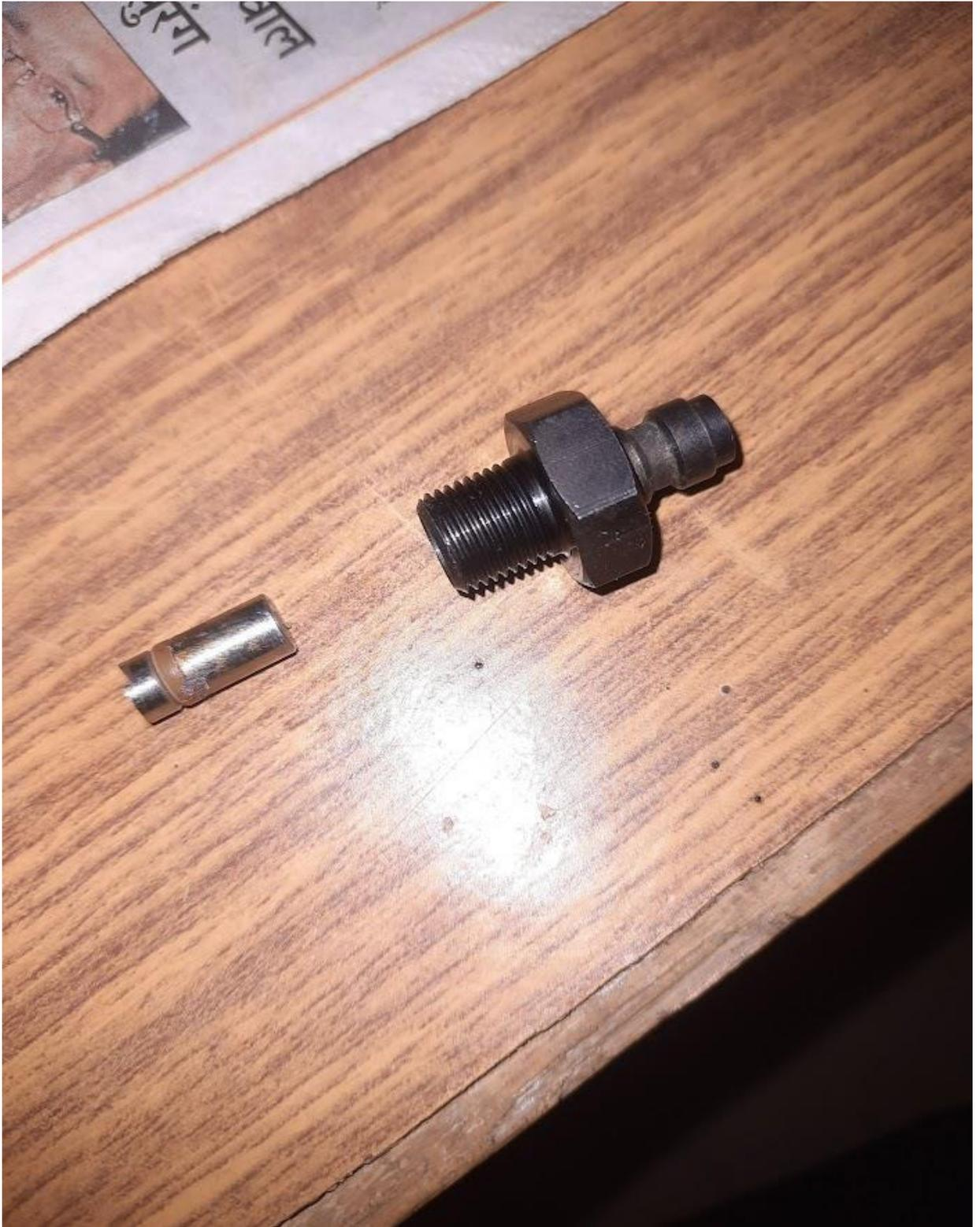
3. **TRANSFER PORT USES 02 XBS 008(N 70) O RINGS ON BOTH SIDES**
