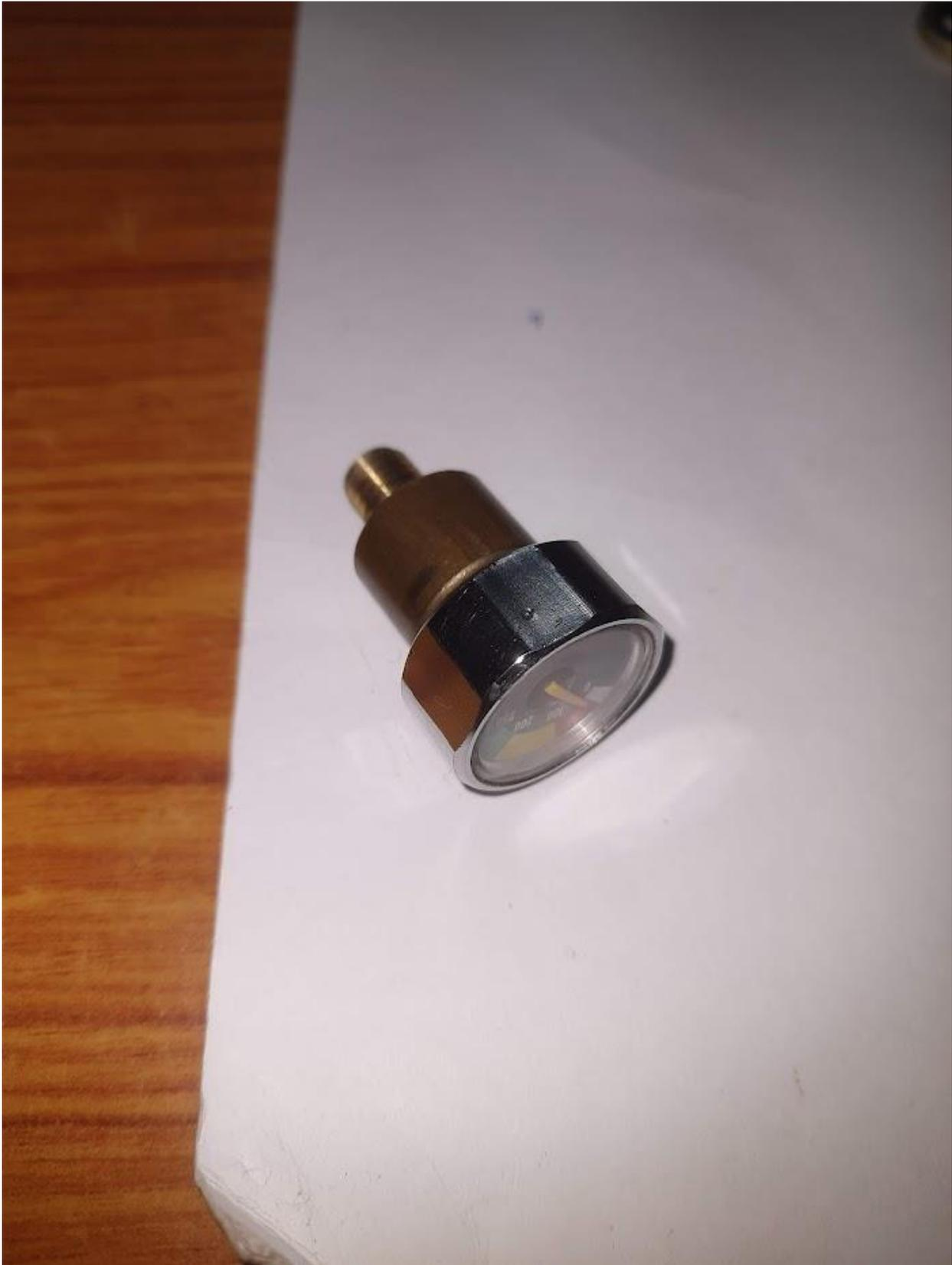
**8 . SLINGSHOT HAMMER BRASS SCREW NEEDS TO BE SCREWED WITH INNER SILVER COLOR HAMMER USING LOCTITE(only if disassembled)**
