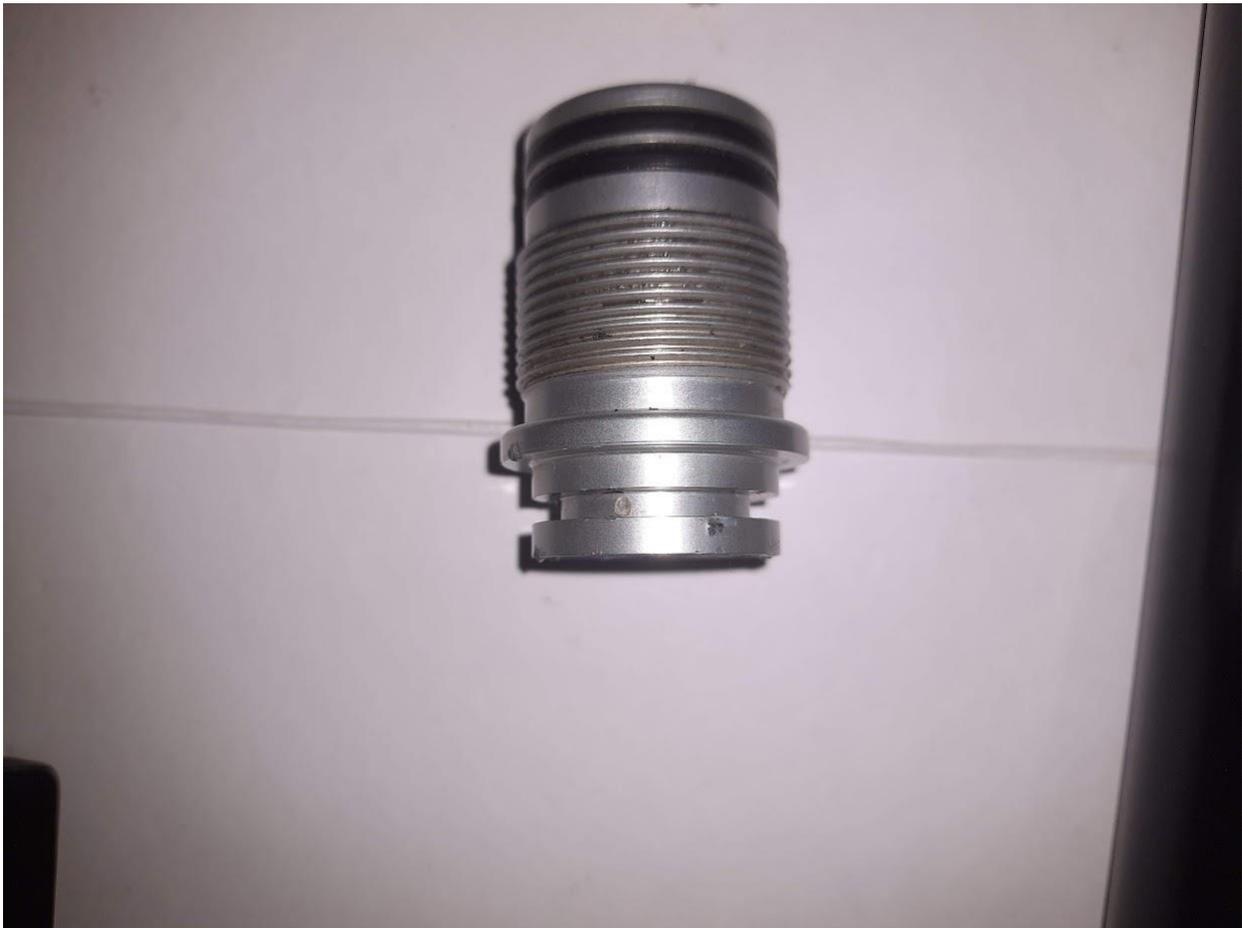
2. 01 X BS 006(urethane) O RING AND 01X 1/8 DOWTY SEAL FOR FILL PORT PISTON
