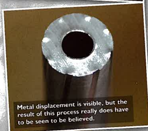
...after an industrial strength squeeze, the Smooth-Twist barrel emerges.
