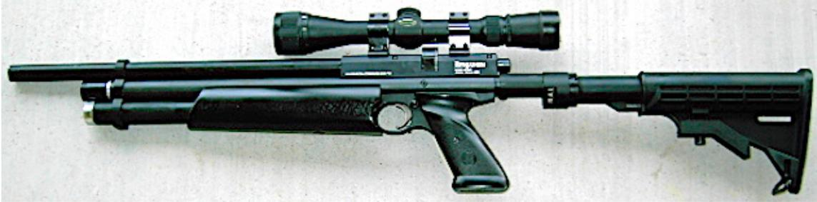
*This P-Rod was converted to twin (chamber) tube, had a B Staley tune, a shroud extension and a Mad Dog AR-style telescoping shoulder stock.*
