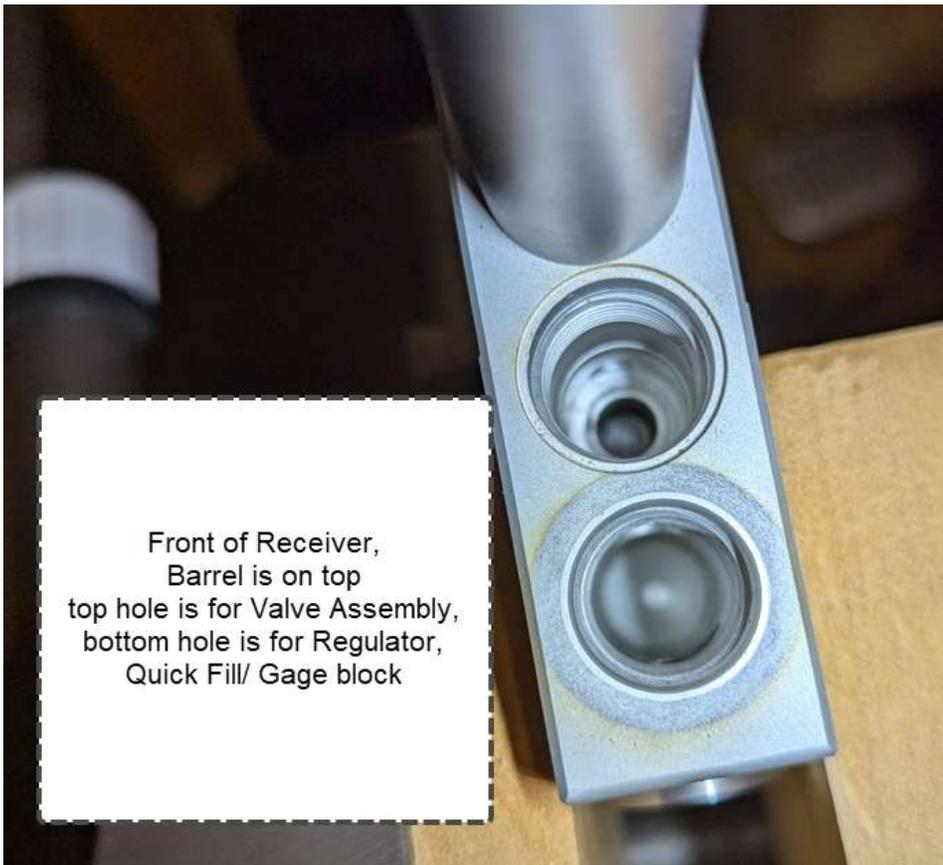
If Valve body does not fall out of receiver block, use a wooden dowel or Allen wrench to push out via the Hammer Assembly chamber.
