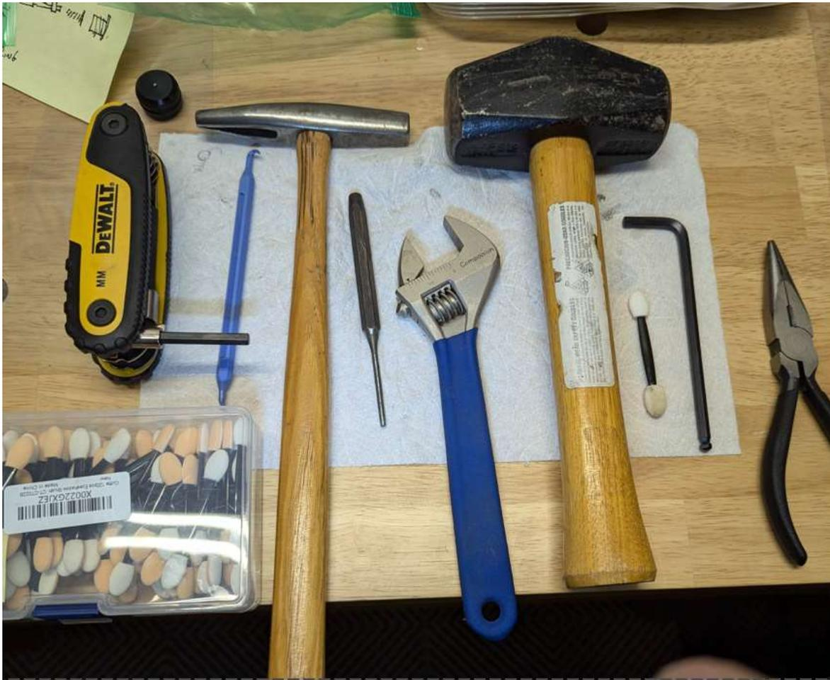
Tools used: 5 mm Allen (blanking Plugs), plastic O-Ring Pick, hammer, punch (trigger pins), spanner wrench, hammer (regulator), eye-shadow sponge (clean), 5 mm Allen, needle nose pliers
