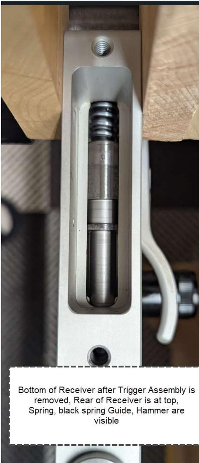
Trigger assembly must be removed before proceeding. Hammer can NOT be removed until Trigger Assembly is removed.
